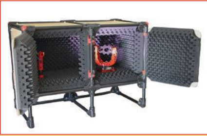
▲ Fig. 1 mmWave and sub-THz antenna test setup.
